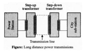
The large-scale transmission and distribution of electrical energy over long distances is done with the use of transformers. The voltage output of the generator is stepped-up. It is then transmitted over long distances to an area sub-station near the consumers. There the voltage is stepped down. It is further stepped down at distributing sub-stations and utility poles before a power supply of 240 V reaches our homes.
